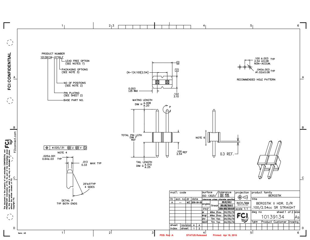
TOTAL PIN LENGTH TAIL LENGTH MATING LENGTH **PRODUCT** DIM G DIM G DIM H DIM F DIM F DIM H NUMBER **INCH** MM **INCH** MM INCH MM 10139134-XYY 0.48 12.19 0.15 3.81 0.23 5.84
