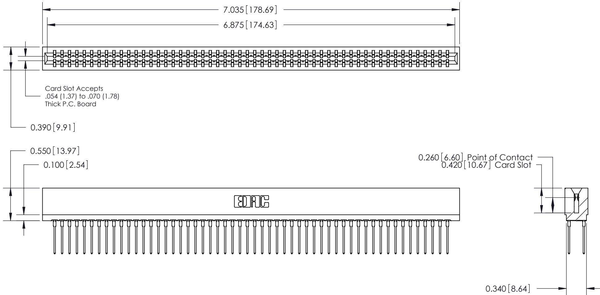
726 Series Ultra-Mate Card Edge Connector - Press Fit
