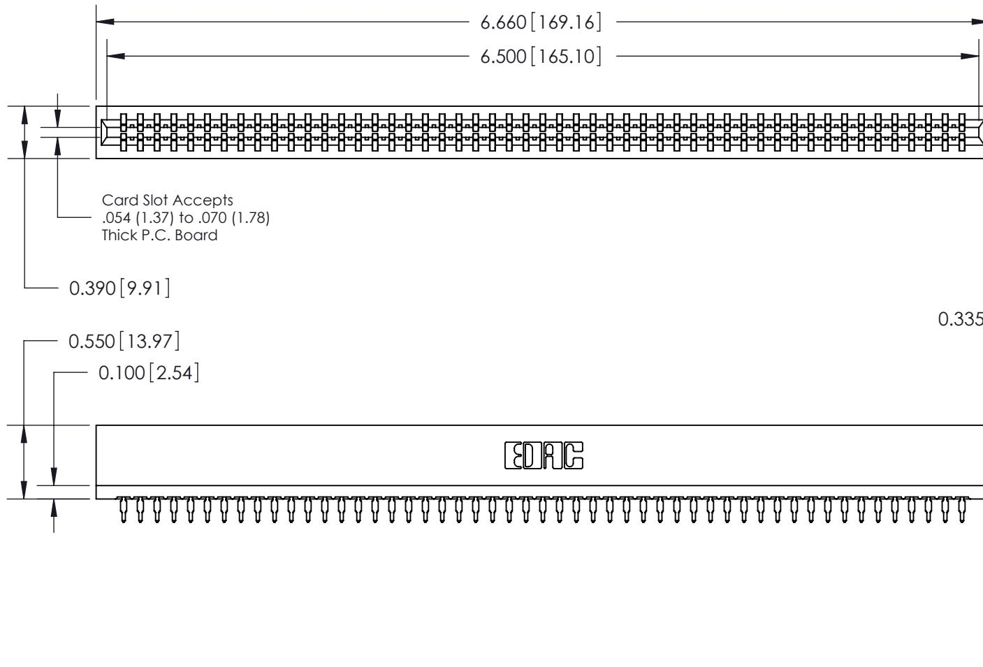
726 Series Ultra-Mate Card Edge Connector - Press Fit
