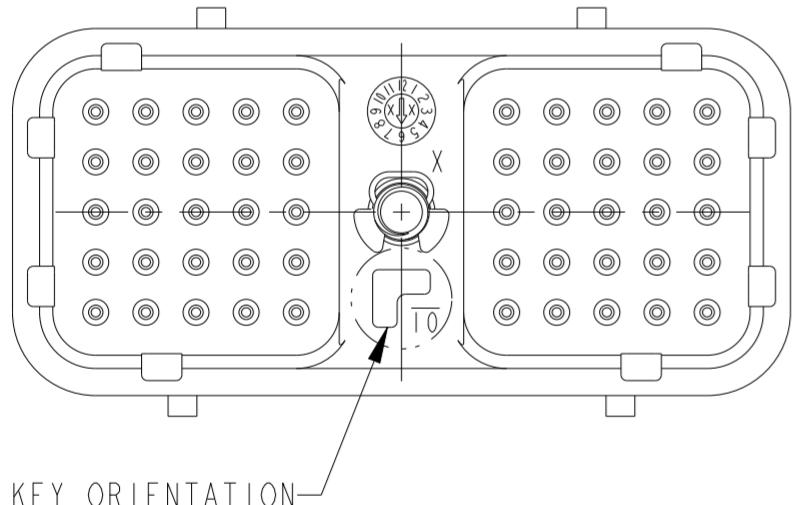
5 MATERIAL: HOUSING: PA46 30% GF (BLACK); BOLT: STEEL, TRIVALENT ZINC PLATED (ROHS COMPLIANT); CLIP: STEEL; GROMMET: VMQ
