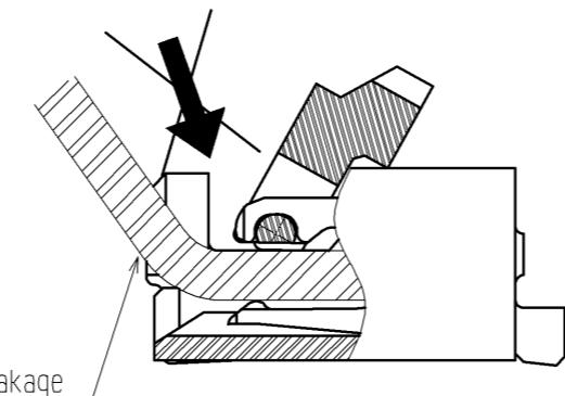
◆Checking the Locking Condition
