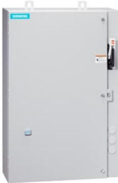
Non-reversing motor starter, Size 1, Three phase full voltage, Solid-state overload relay, OLR amp range 0.25-1A, Combination type, 30A fusible disconnect, 30A/250V fuse clip, Enclosure NEMA type 4/12, Water/dust tight for outdoors, Extra-wide enclosure
