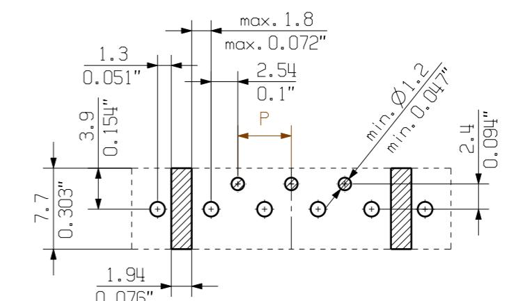
D = 1.5/0.059" (REFLOW SOLDERING)
