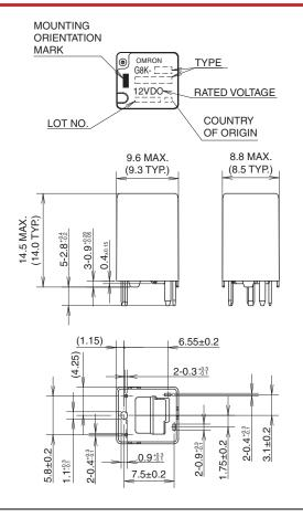
FOR REFERENCE: PCB MOUNTING HOLES (BOTTOM VIEW)
