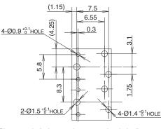
\*Please study & choose other appropriate hole diameters if confirmed the diameter values recommended above don't work with the soldering process.
