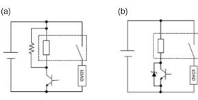
OMRON recommends coil driver circuit (b) and (c) for coil surge suppression. However the circuit (d) is not recommended because it may negatively affect the durability performance.
