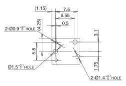
\*Please study & choose other appropriate hole diameters if confirmed the diameter values recommended above don't work with the soldering process.
