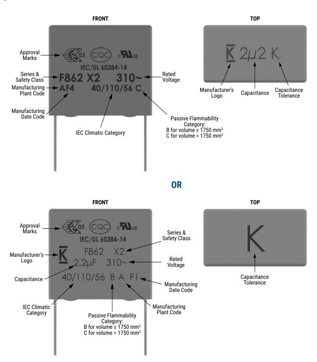
Slight change in the layout can be possible but this does not affect the content of the information of the current marking.
