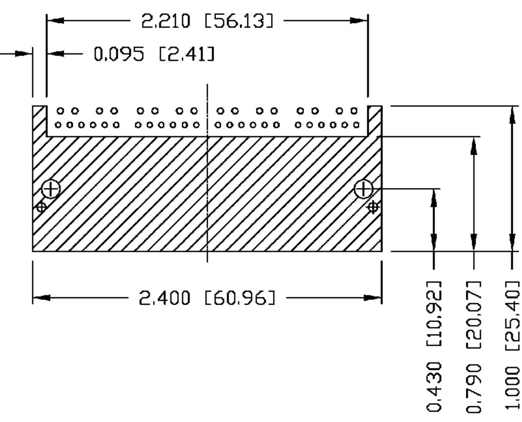
THE SHADED AREA ON THE CUSTOMER BOARD ARE RECOMMENDED TO BE CLEAR OFF ANY VIA HOLE OR COMPONENT PAD.
