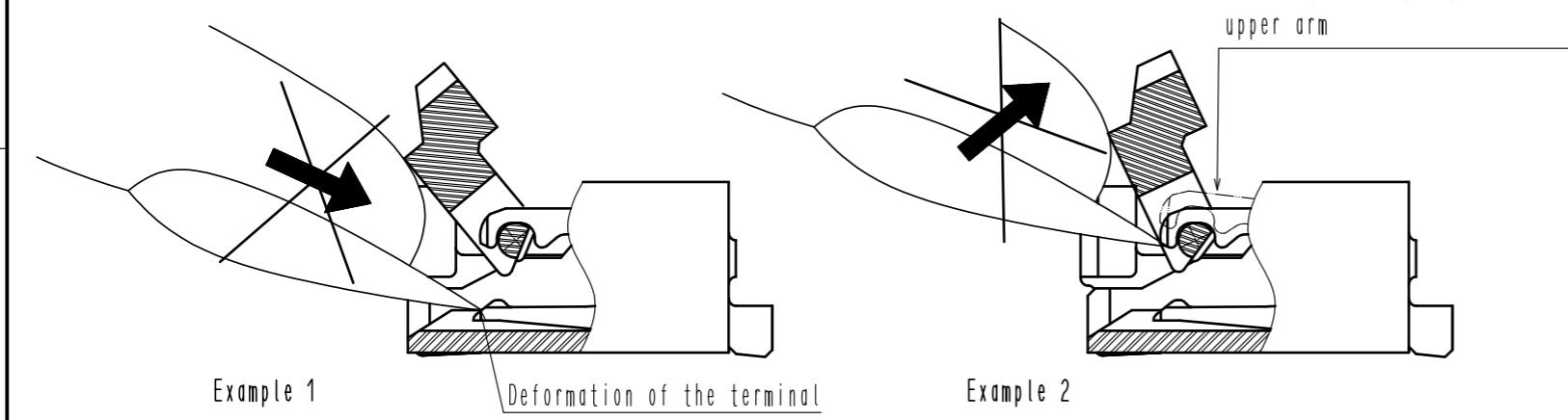
2. The actuator rotates around the rotational axis as shown below.
