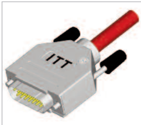
Assemble the other half (screwing force: 100-120 Ncm)
