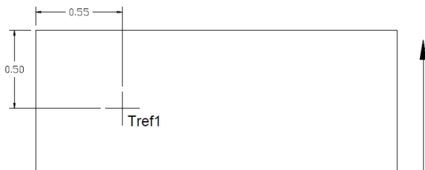
Figure 18. Case ( T_{REF} ) Temperature Measurement Location (top view).
