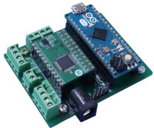
Figure 2. ONBB4AMGEVB Board with Arduino Micro and LV8714TASLDGEVB Board
