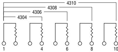
These models incorporate 2, 3, 4 or 5 isolated thick-film resistors of equal value, each connected between two pins.
