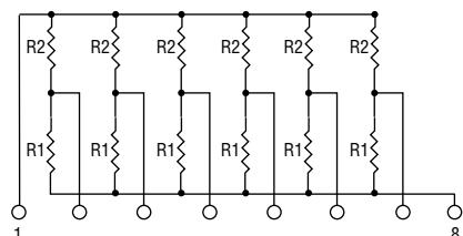
4308M-104 (shown above) is an 8-pin configuration and terminates 6 lines. Pins 1 and 8 are common for ground and power, respectively. Twelve thick-film resistors are paired in series between the common lines (pins 1 and 8).
