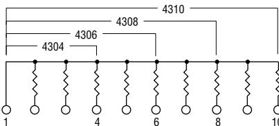
These models incorporate 3, 5, 7, or 9 thick-film resistors of equal value, each connected between a common bus (pin 1) and a separate pin.
