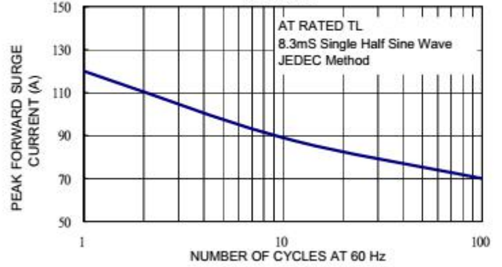
FIG. 2 MAXIMUM NON-REPETITIVE FORWARD SURGE CURRENT
