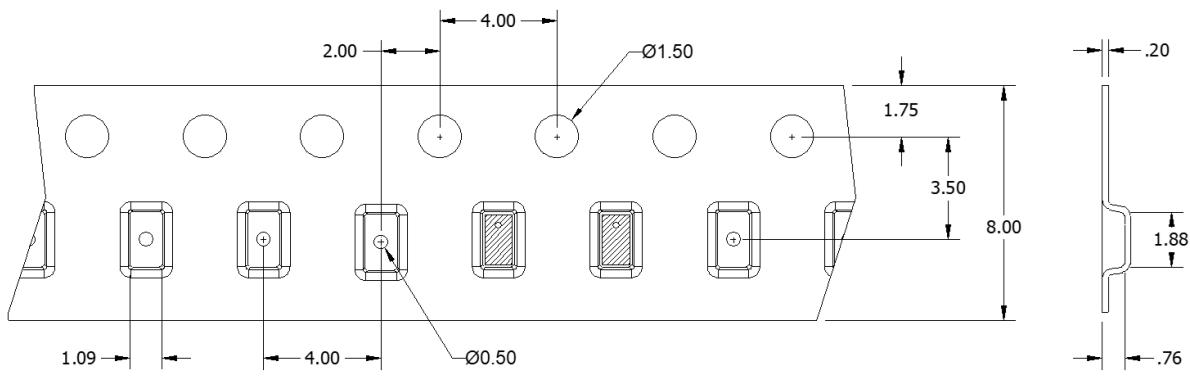
Dimensions are in Millimeters
