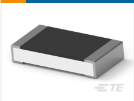
TE Part #4-2176391-7 RQ 1206 37K4 0.1% 10PPM 5K RL
