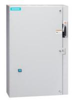
Non-reversing motor starter, Size 2 1/2, Three phase full voltage, Solid-state overload relay, OLR amp range 25-100A, Combination type, 100A non-fusible disconnect, Enclosure NEMA type 1, Indoor general purpose use, Extra-wide enclosure
