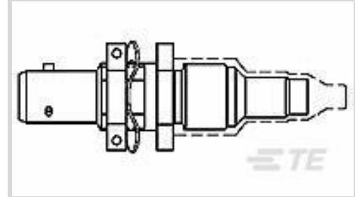
Data Bus Connector Type: **Jack**Data Bus Connector Style: **Bayonet**Polarization (Bayonet Style): **C**Data Bus Connector Contact Type: **Socket**
