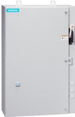
Non-reversing motor starter, Size 1 3/4, Three phase full voltage, Solid-state overload relay, OLR amp range 10-40A, 208VAC 60Hz coil, Combination type, 60A non-fusible disconnect, Encl NEMA type 4X 304 S-Steel, Water/dust tight noncorrosive, Extra-wide enclosure
