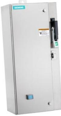
Non-reversing motor starter, Size 1 3/4, Three phase full voltage, Solid-state overload relay, OLR amp range 10-40A, Combination type, 60A fusible disconnect, 60A/600V fuse clip, Encl NEMA type 4X 304 S-Steel, Water/dust tight noncorrosive, Standard width enclosure
