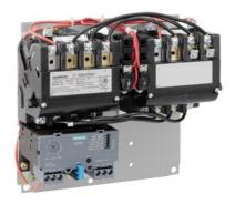
Reversing motor starter Size 1 3/4 Three phase full voltage Solid-state overload relay OLRelay amp range 10-40a 110-120/220-240VAC 60HZ coil Noncombination type Enclosure type (open)
