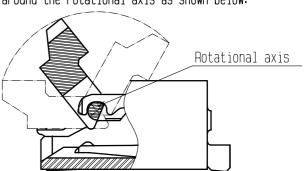
3. The actuator will not open more than 120°. Do not apply any force backward beyond this point. Otherwise, the actuator may come off or break.
