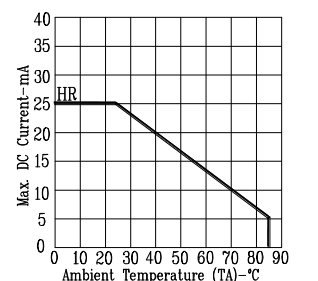
Fig5. MAX. ALLOWABLE DC CURRENT VS. AMBIENT TEMPERATURE.
