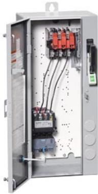
Non-reversing motor starter, Size 0, Three phase full voltage, Solid-state overload relay, OLR amp range 0.75-3.4A, 110V 50Hz / 120V 60Hz coil, Combination type, 30A non-fusible disconnect, Enclosure NEMA type 4/12, Water/dust tight for outdoors, Standard width enclosure
