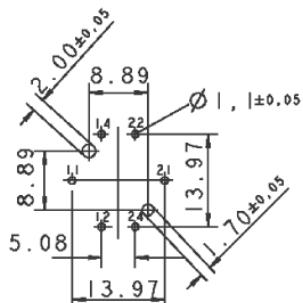
PCB hole pattern, component side
