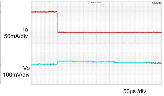
Figure 11. Transient Response ( T_a=-40^\circ\text{C} ) ( I_o = 0.1\text{A} \rightarrow 0\text{A} )
