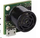
to integrate many sensors into one system and experience little to no effect from the sensor to sensor interference that can occur with other ultrasonic sensor solutions. The USB-ProxSonar-EZ features a True/False output and an optional range output. With the USB interface, deploying a network of ultrasonic sensors has never been easier. \*Factory calibration and testing is standard.
