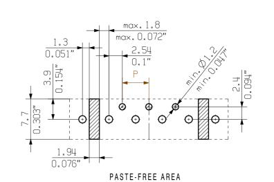
D = 1.5/0.059"(REFLOW SOLDERING) RECOMMENDATION FOR AUTOMÁTIC ASSEMBLY
