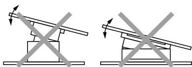
■ Keep the PC board warp no more than 0.03 mm in relation to the overall length of the connector.
