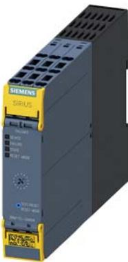
fail-safe direct-on-line starter, 3RM1, 500 V, 0.09 - 0.75 kW, 0.4 - 2 A, 24 V DC, spring-loaded terminal (push-in)
