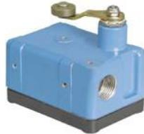
**Enclosed Switch Series OP: Side Rotary, Fixed lever length with steel roller, 1NO 1NC Snap Action SPDT, CW or CCW actuation, No return lever, No mounting bracket furnished**
