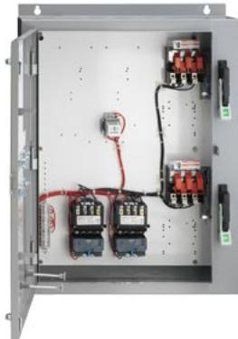
Pump control panel, Duplex controller NEMA size 0 Solid-state overload relay, OLR amp range 3-12A, 120 VAC coil, Fusible disconnect HOA Sel Sw. and Start P.B., Enclosure NEMA type 3/3R,12 Weather proof outdoor use
