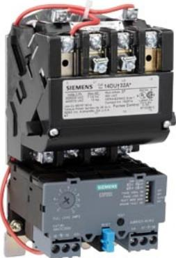
Non-reversing motor starter Size 1 Three phase full voltage Solid-state overload relay OLRelay amp range 3-12A 110VAC 50HZ / 120VAC 60HZ coil Combination type No enclosure
