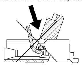
3. Do not rotate the actuator when FFC/FPC TAB is on right and left guides for positioning FFC/FPC. Make sure the position of FFC TAB and guides before rotate the actuator.
