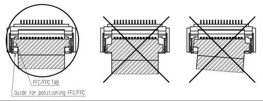
♦ Checking the Locking Condition
