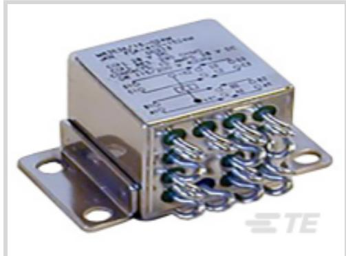
Contact Arrangement: **4 Form C, 4PDT, 4 C/O**Terminal Plating: **Tin-Lead**Contact Current Rating (Max): **10 A**Coil Voltage Rating: **6 VDC**Coil Resistance: **18 Ω**
