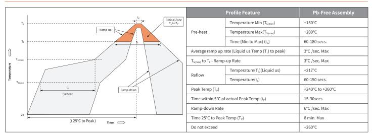
Note 1: All temperature refer to topside of the package, measured on the package body surface.
