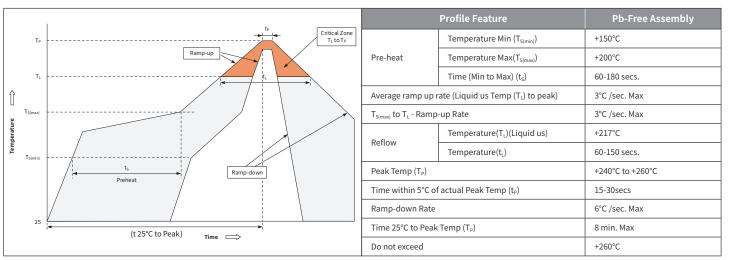
Note 1: All temperature refer to topside of the package, measured on the package body surface.
