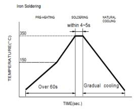
Iron Soldering times: 1 times max.
