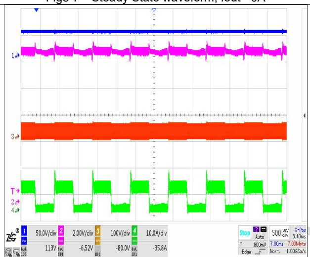
1#:Vin 2#:Vout 3#:Vsw 4#:IL Vin=48V Vout=12V/1-9A Fig8-9 Load Transient Ripple
