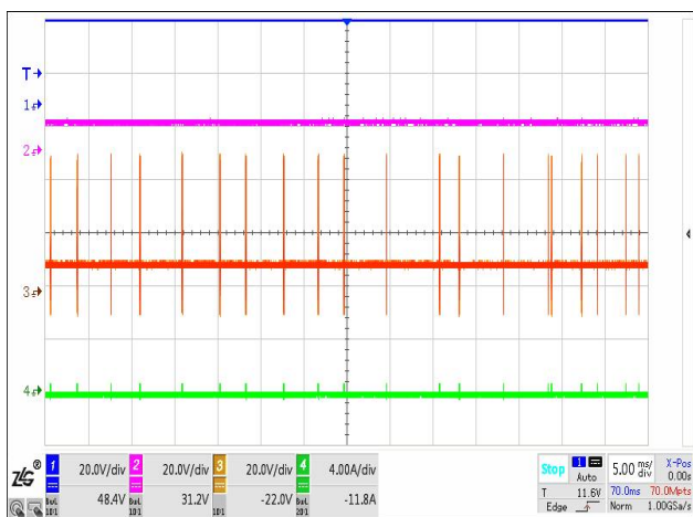
1#:Vin 2#:Vout 3#:Vsw 4#:IL Vin=48V Vout=12V Fig8-7 Steady State waveform, Iout =0A
