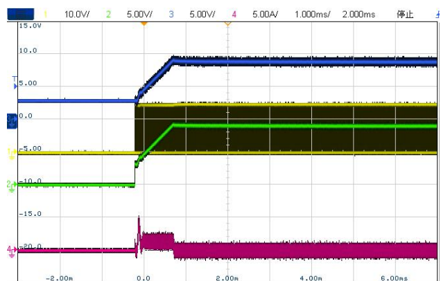
CH1:SW1 CH2:SW2 CH3:Vout CH4:IL
