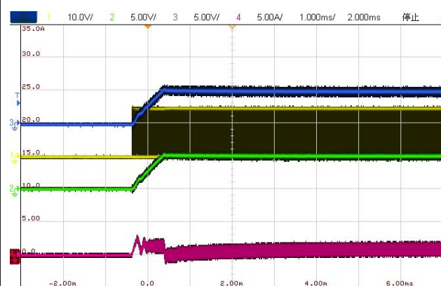
Fig.8-4 Start up waveform, Iout =0A
