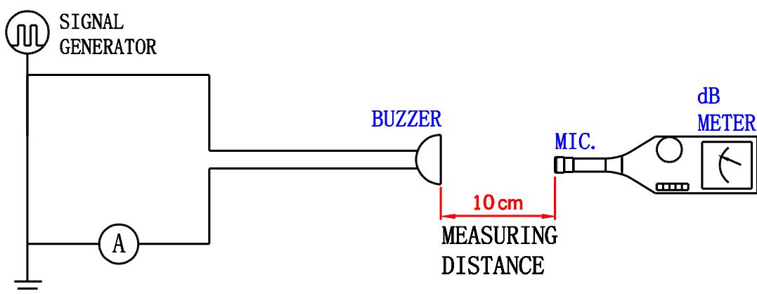
**In the measuring test, buzzer is placed as follows:**
