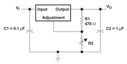
$<sup>^*</sup>$  =  $C_{IN}$  is required if the regulator is located near power supply filter.
