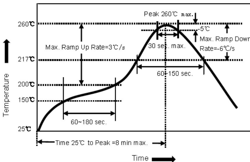
\*Above reflow soldering curve is from J-STD-020D.
