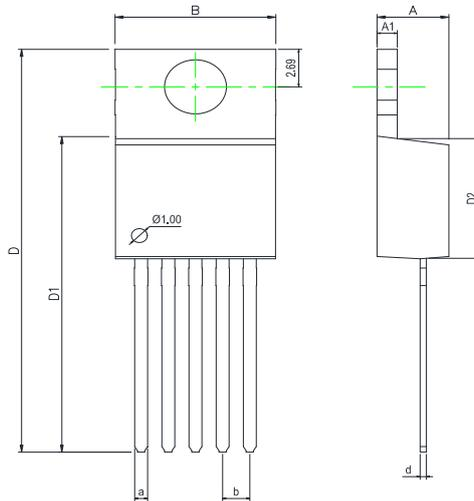
Dimensions In Millimeters(TO-220-5)
