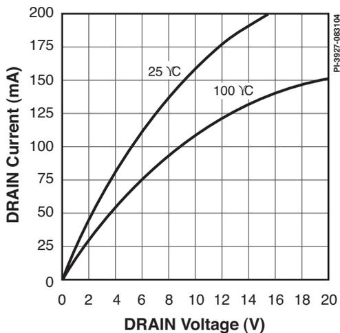
Figure 8. Output Characteristics.
