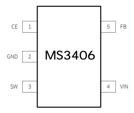
The package of MS3406 is SOT23-5L, with pin assignment shown in following ta ble:
