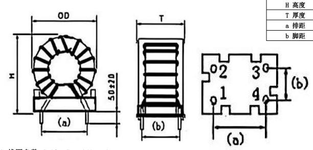
2. 线圈参数 Coils Specification: 绕组结构线径和匝数 Connection and Turns and Wire
