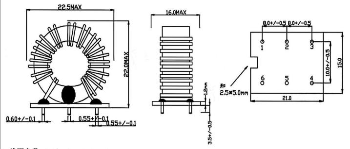
2. 线圈参数 Coils Specification 绕组结构线径和匝数 Connection and Turns and Wire
